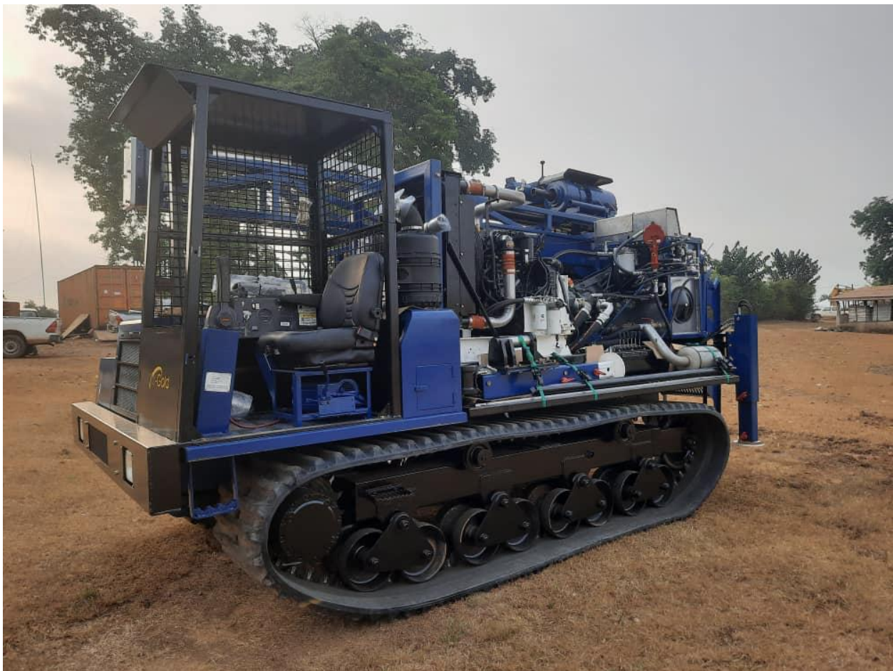
(Picture of Xtra-Gold's CS1000/P4 Crawler-Mounted Diamond Drill Rig Arriving at Our Mine Camp in Ghana)
