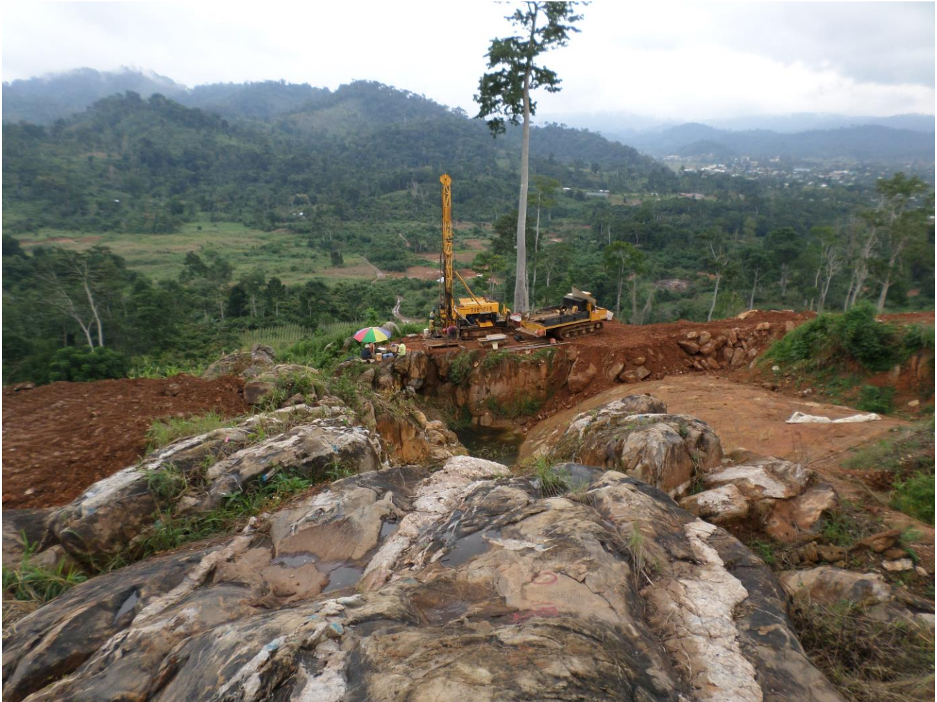
Diamond core drilling on High-Grade Shoot discovery outcrop at Cobra Creek Gold Corridor shear system (2016)
